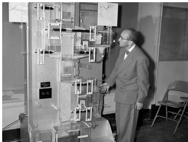
Fig. 1: The MONIAC IS/LM model Source: Smithsonian Magazine [Fe2014]
